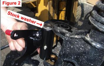
Bolt the new spindles to the cart using the stock kingpin, nut, and washer.
