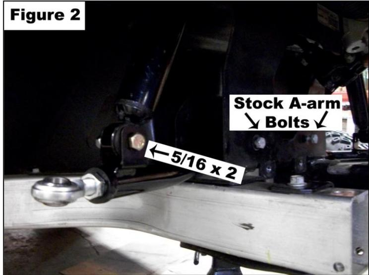
10. Using a 3/8" drill bit and the center hole of the sub-frame as a guide drill through the frame of the cart.
