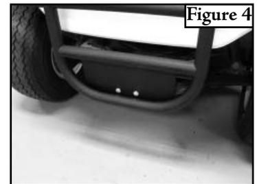
4. Install the brush guard in place of vacated A-Arm bolts (Figure 4).
