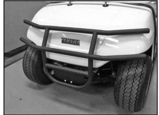
1. Remove the front bumper from cart, save the two bolts from the bumper for future use (Figure 1).
