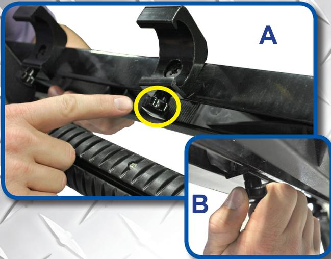
A) Loosen threaded knob on bottom of rail attachment and slide Golf bag holder onto rail.
