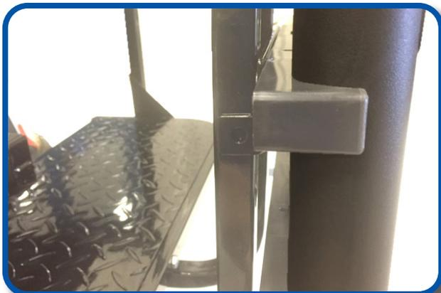
Place rod holder w/bracket on outside of grab bar at desired height.
