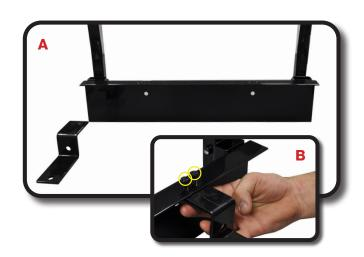
Place and center your assembled bagwell bracket for installation. Mark locations in bagwell. Using a 15/64 Drill bit, drill holes through bagwell and underlying frame.
