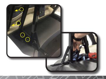
Install rear struts to front side of tabs on main support brackets, using retained hardware from Step 3.
