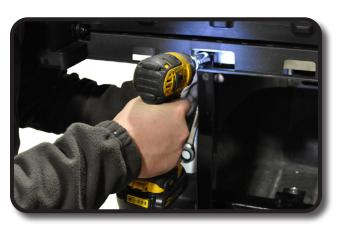
A) Using 3/8" drill bit with light pressure, slowly drill through back bumper as shown.
