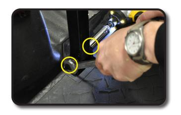
Attach grab bar to foot rest using additional hardware from Pack 6.
