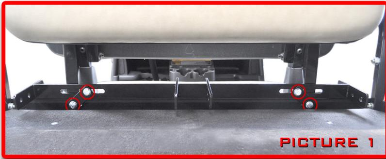
For the EZ-Go RXV, place seat belt bracket on top of the rear seat frame as shown in picture 1.
