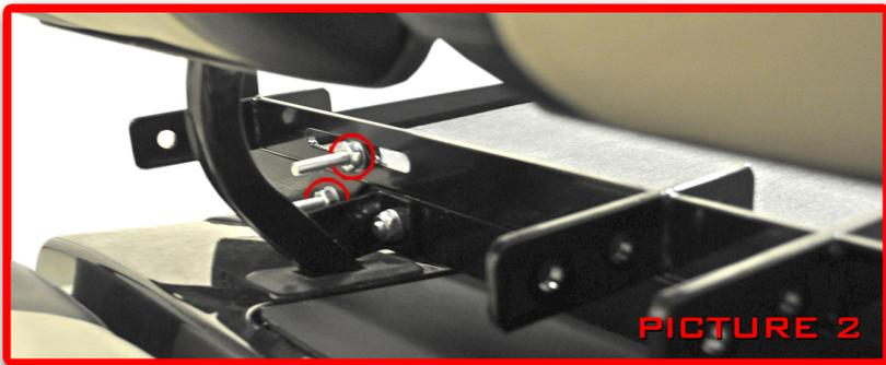
Using mounting brackets, attach seat belt bar to seat frame using hardware provided and tighten as shown in picture 2.
