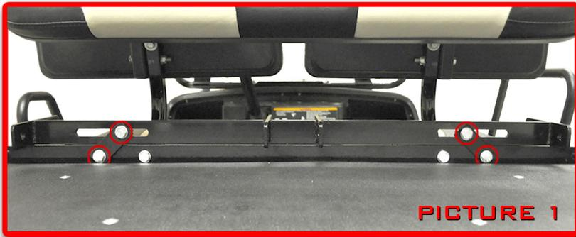
For the Yamaha G-Series, place seat belt bracket on top of the rear seat frame as shown in picture 1.
