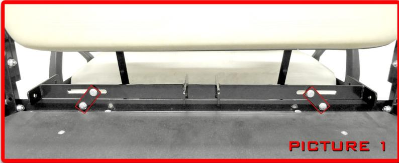
For the Club Car DS, place seat belt bracket on top of the rear seat frame as shown in picture 1.
