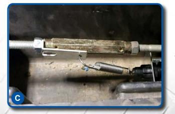
Loosen lock nut on brake rod. Place the forked bracket around the brake rod behind the lock nut and tighten the lock nut sandwiching the bracket. Place the brake switch on the floor of the car with the spring running towards the back of the car to the brake switch.
