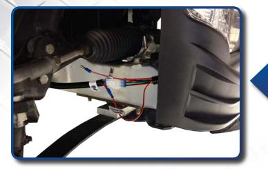
Route the 6 pin headlight connector through the cutout in the passenger dash.
