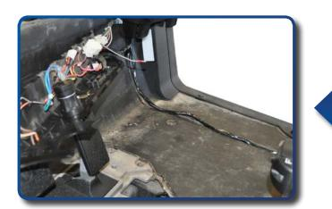
From the battery compartment, route the 12-pin connector portion of the new harness along the floor channel on the passenger side of the vehicle to the dash.
