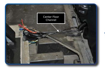
From the battery compartment, route the brake light accessory wires through the center floor channel that leads to the brake compartment. Remove the console screws. Retain hardware.
