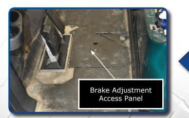
Remove all screws securing floor mat to the vehicle. Retain hardware. Remove floor mat.
