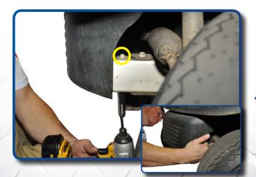
Remove factory bumper by removing the two factory bolts located in the frame. Retain hardware.
