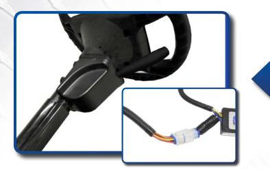
Attach horn to orange and black female spade connectors and secure horn to metal frame under front cowl using supplied hardware.
