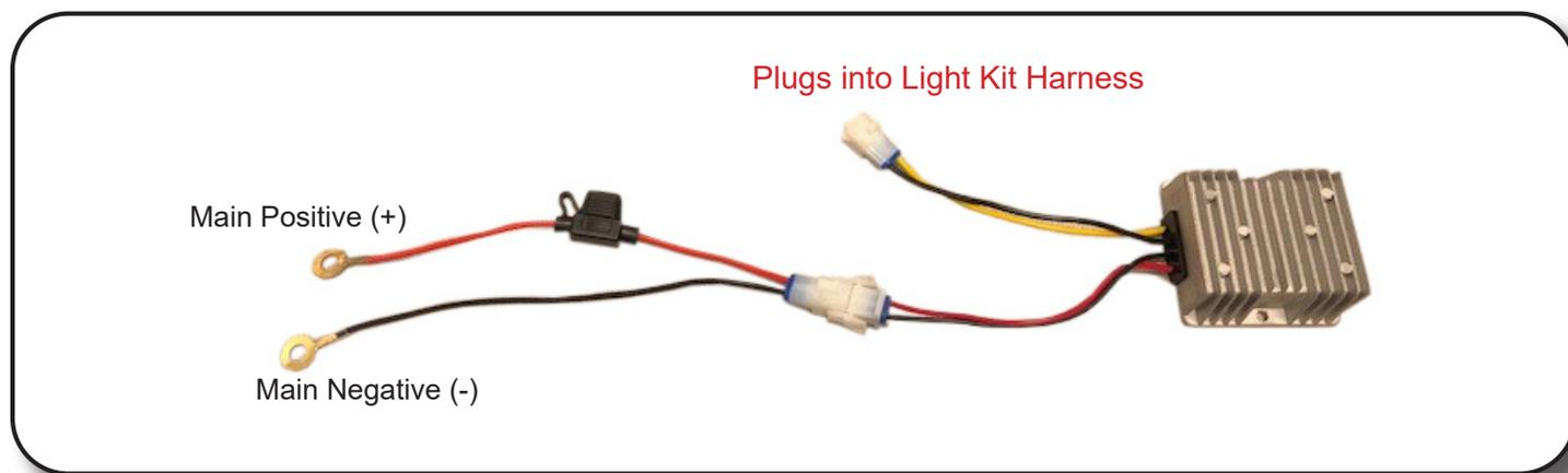
The voltage converter included must be used on all carts electric and gas. Connect the red wire with the fuse to the Main Positive terminal of the battery pack. Connect the black wire to the Main Negative terminal of the battery pack and tighten hardware.
