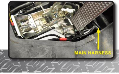
Red plugs should be aligned to passenger side, white plugs for driver's side.
