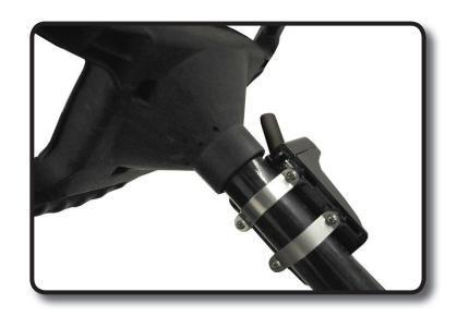
Attach turn signal back cover to turn signal assembly.
