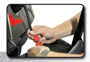
Install new tail lights using retained hardware.
