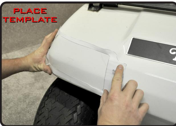
Draw the inside of the template out with a writing utensil. Next drill a pilot hole so you will have a starting point to begin cutting.
