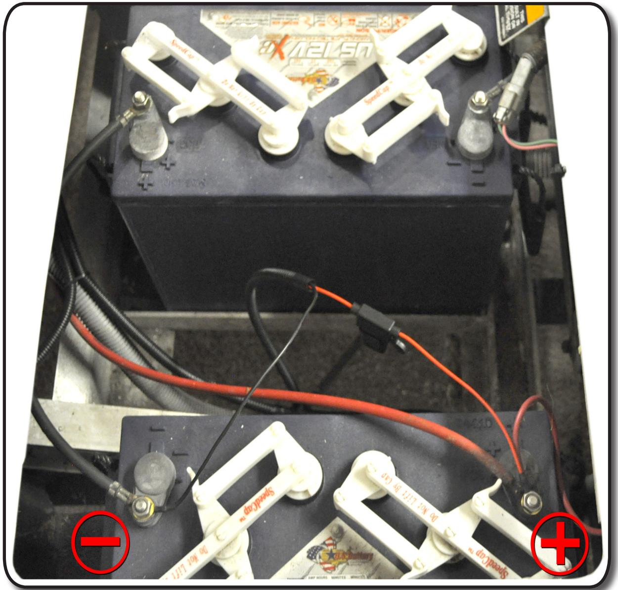
If you have 12 volt batteries wire the harness to the battery as shown. If you have 8 Volt batteries a 16/12 voltage reducer will be necessary.
