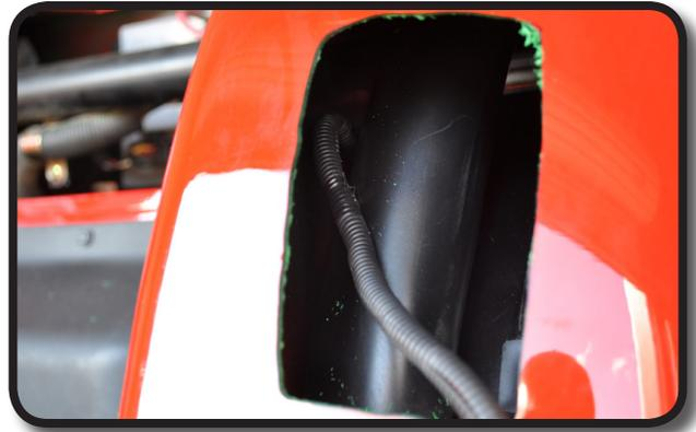
Use the supplied zip ties to fasten wiring harness to vehicle. We recommend fastening the wiring harness to frame members in the front of the vehicle in order to prevent the harness from making contact, rubbing, or being pinched by moving parts, such as the suspension. Use two zip ties to tie the wiring harness to the frame at the back of the motor compartment as shown. Replace motor cover.
