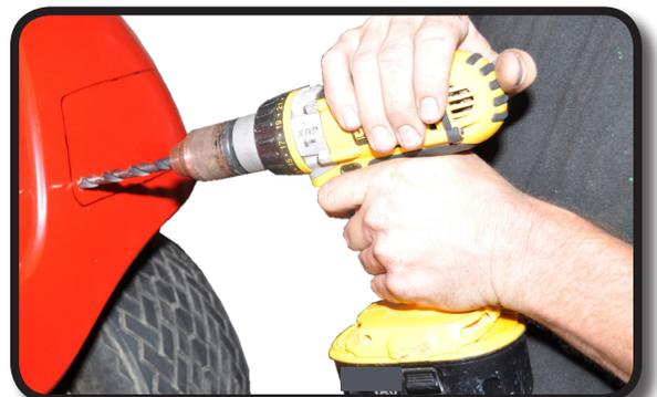
Cut out bodywork. **IMPORTANT:** As you approach the top of the cut, back out the cutting tool to prevent cutting into the fender well. Cut the cowling to the inside of the mark.
