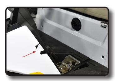
Place the cowl on a flat surface and use something to prevent scratching. Then remove factory Headlight push nuts, by *gently* prying them off with needle nose pliers to avoid damage.
