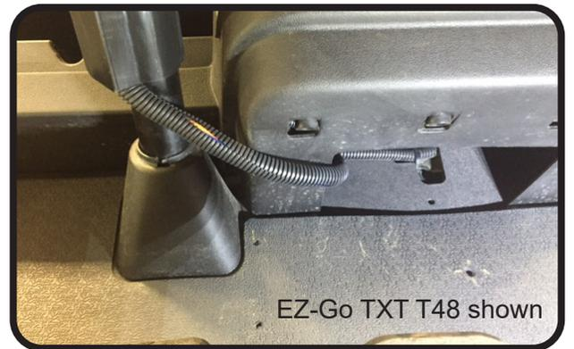
Connect 9 pin from **Control Box** harness to 9 pin connector of **GTW Upgrade Harness** from GTW light kit.
