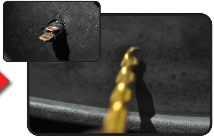
Attach Blue and Yellow wires from Control Box Harness to **Hazard Switch** as shown. There is no wire orientation required, wires can attach to either post.
