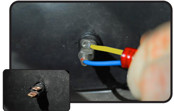
Attach **Horn** to purple and black female spade connectors from your light kit Upgrade Harness and secure horn under front cowl.
