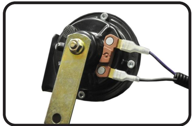
For the **Brake Pad**, plug the male and female bullet connectors together from GTW Upgrade Harness and **Brake Pad** as shown.
