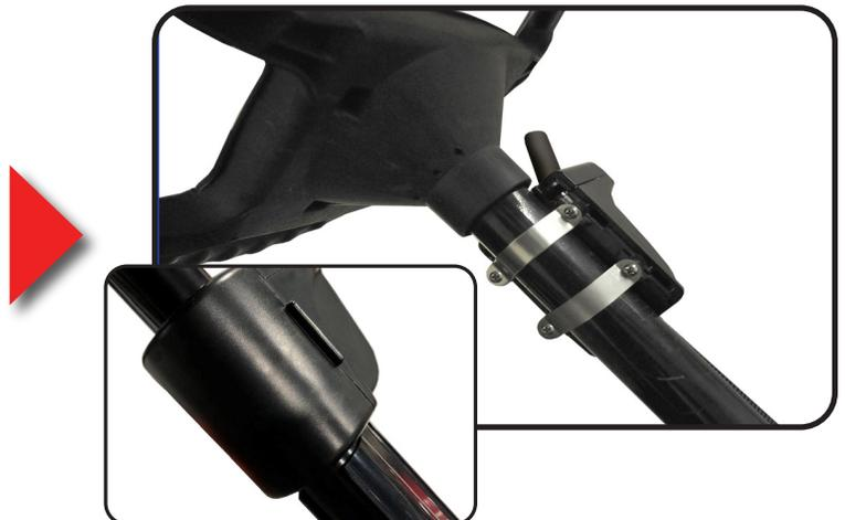
Attach **Column Cover** to steering column, secure harness in column cover chase.
