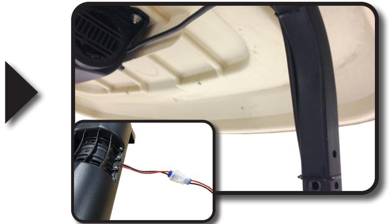
**The voltage converter included must be used on all carts electric and gas. Use the converter on gas carts to prevent Starter Generator voltage spikes that could cause damage to fan motor. Failure to use converter will cause damage to the fan and warranty will not apply.**
