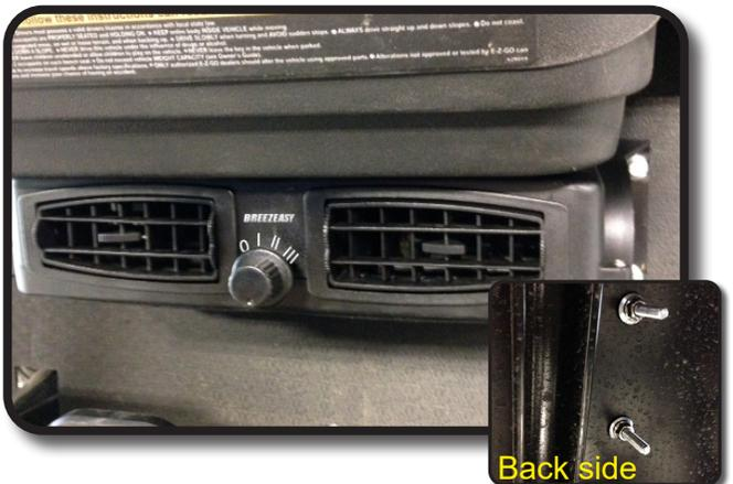
**NOTE:** DO NOT overtighten hardware as this can cause damage to brackets and floor.
