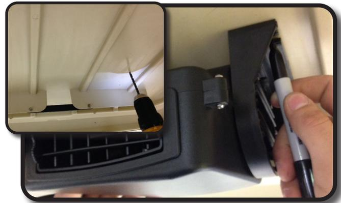
Insert the four 6mm x 45mm bolts through the top of the roof with rubber side of washer down as shown. If you are installing the fan on a TXT the four 6mm x 70mm bolts are needed.
