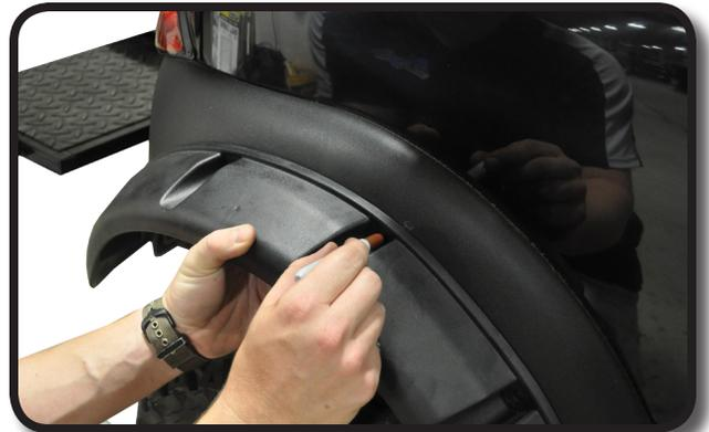
Drill first hole using a 9/32" drill bit. Ensure area behind body work is clear to avoid potential damage to wiring or other bodywork.
