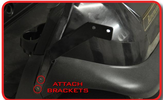
Attach clays basket to brackets on both sides using hardware pack.
