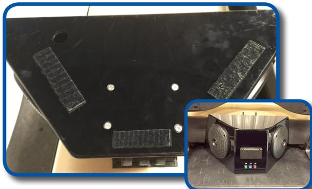
Attach supplied fastening tape to the speaker box as shown. Now peel film off bottom side fastening tape. This will secure box to car. Use a tape measure to find center point of car and attach box.
