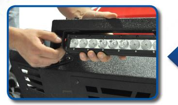
Make adjustments to tabs for the light bar to fit inside of and tighten brackets.
