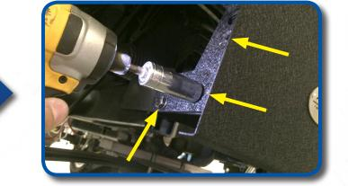
Before tightening the bumper, you can adjust the bumper to your specifications by using the slotted holes in the bumper and bracket. Once bumper is adjusted to your preferred location you may tighten all hardware.
