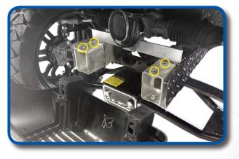
Remove factory bumper from cart by taking out two bolts from back of bumper as shown, retain hardware. Also unplug headlight bar if installed on cart.
