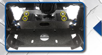
Place the Armor Bumper mounting bracket in place of the factory bumper. Attach using supplied 8mm hardware and two bolts retained from step 1. Tighten.
