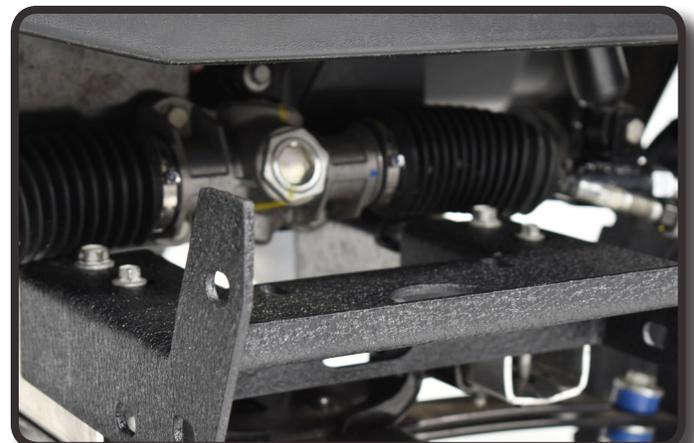
**STEP 4** Using supplied bolts, washers, lock washers, and nuts, attach the Brushguard to the Mounting Bracket as shown.
