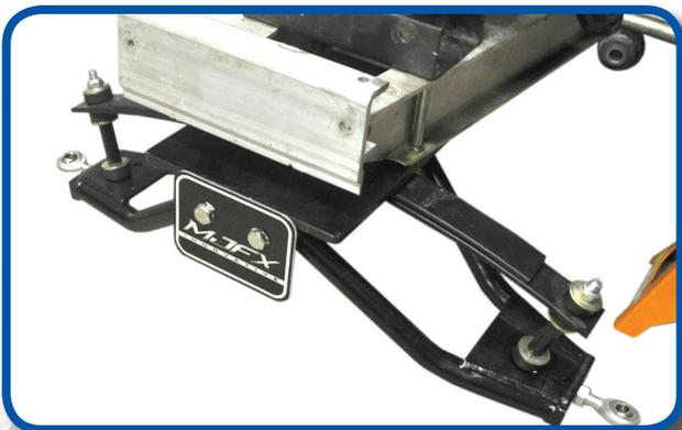
Attach the Main Suspension Assembly using hardware retained from Step 9 and tighten. \*A floor jack is recommended to help hold suspension assembly in place while you get the bolts started.
