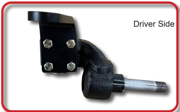
Note the Tie Rod Mount arm angles to the inside of the cart and the spindle is marked which side (P-pass, D-driver).
