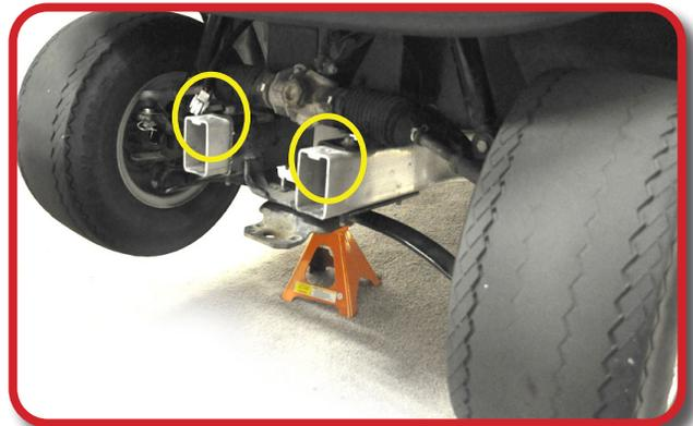
Using a 19mm Socket remove front wheels.
