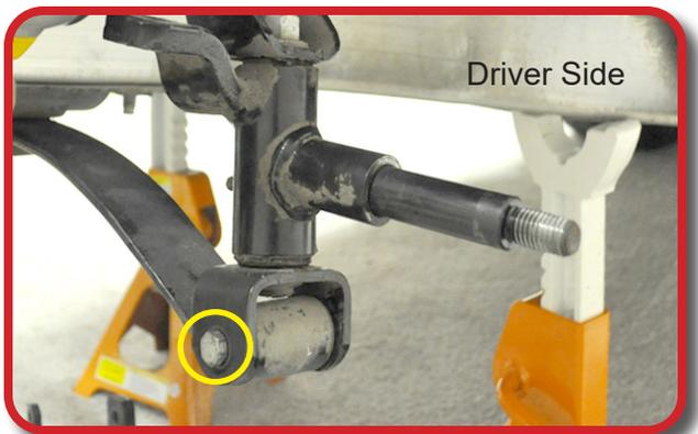
Remove the front spring & plate with a 1/2" Socket. Retain spring plate & hardware, discard spring.
