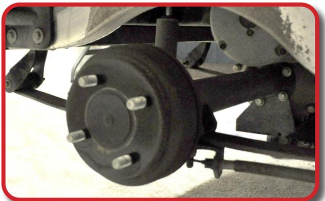
**NOTE:** It is highly recommended to use rear Heavy Duty Leaf Springs if installing a seat kit or cargo box on the rear of your golf cart. The shackle extensions will not be enough to support the weight and will cause too much stress on the single leaf factory spring.
