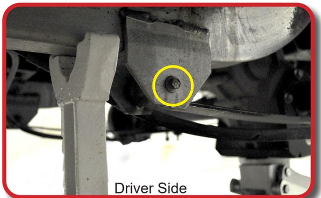
Use jack to lower axle and motor assembly. Reinstall leaf spring on top of axle using hardware retained from Steps 22 and 23. **Torque spring mounting bolts to 18.5 ft·lb (25 N·m)**
