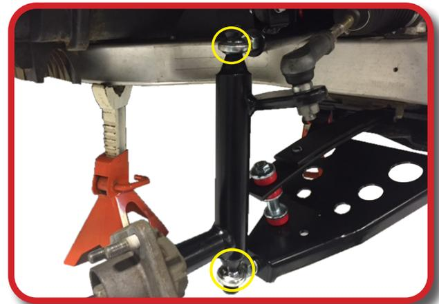
Attach tie rods to new Spindles using retained nut and cotter pin from step 6.
