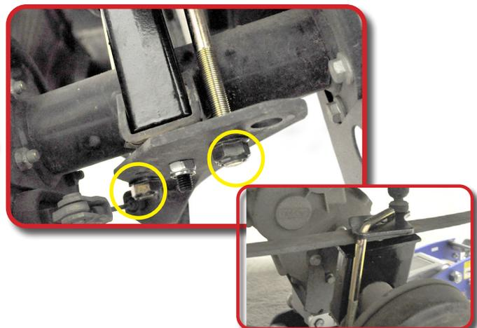
Repeat steps 21-27 on passenger side, use jack to lower axle and motor assembly as needed.
