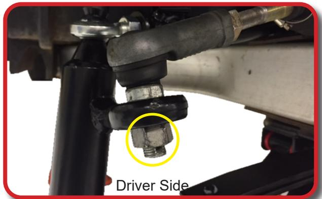
Using a 13mm Socket and Wrench, attach shock to **A-Arm** using the two 8x50mm Hex bolt, four 8x15mm flat washers and two 8mm locknuts.
