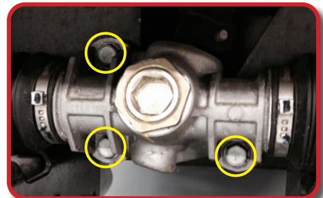
Using a 1/2" Socket remove & discard the factory A-Arms, keep mounting bolts for new A-Arms.
