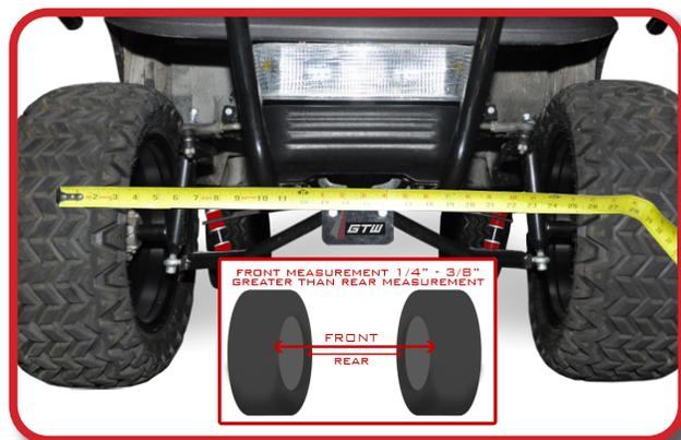
Ensure the wheels are pointing straight forward. To adjust Toe, find a common point to measure from on the inside front and inside rear of the front tires. Adjust until the front measurement is 1/4" to 3/8" greater than the rear measurement.
