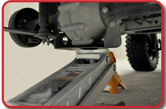
Using a 5/8" Socket remove the driver side U-Bolts. Once the U-Bolts are removed you can remove the lower bushing and hardware from shock using a 9/16" Socket.
