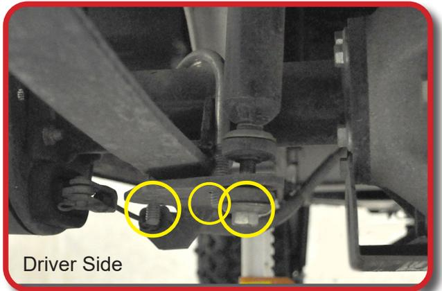
Using a 10mm socket and 13mm wrench remove hardware from rear leaf spring mount. Retain hardware.
