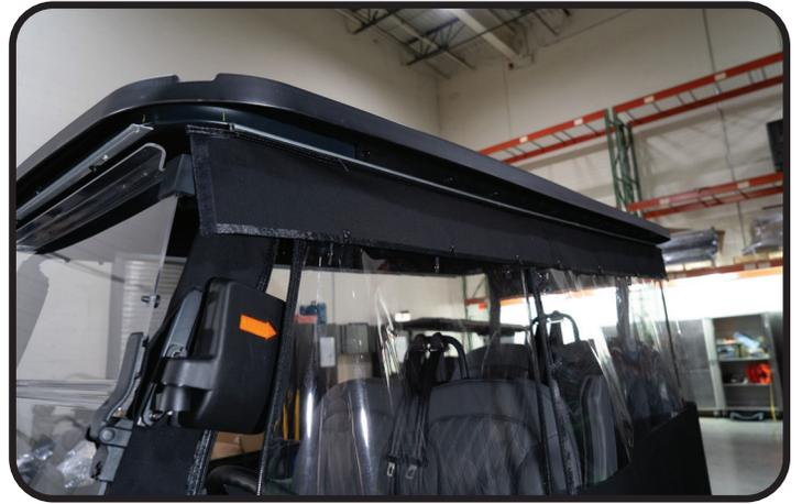
**Note:** When installing side and rear panels, make sure excess panel is held even with track to avoid binding when sliding panel into track.
