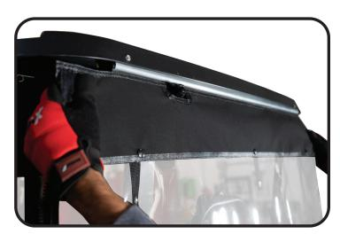
In order to install the windshield, mark the OEM mounting hole location on top of the front strut cover. Cut a very small "X" with a razor knife to allow windshield hardware to feed through. Install windshield, and insert windshield hardware through the hole in the strut cover and into the strut.
