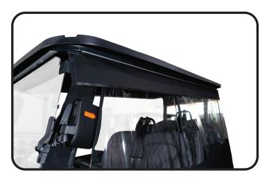
Note: When installing side and rear panels, make sure excess panel is held even with track to avoid binding when sliding panel into track.
