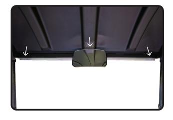
Install the side tracks. There are two pieces of track per side. Starting at the front of the top, orient the track so that the track slot is on the outside. Align one of the metal tracks to the length of the top. Using a measuring tape and marker, if necessary, mark two holes where you will secure the top to the track. Secure the track to the top using the provided self-tapping screws.
