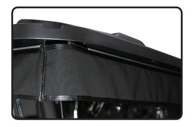
Now that all pieces of the enclosure are installed on the cart, ensure the enclosure and valences are properly aligned to match cart body lines. When satisfied, zip all corners of the enclosure, and attach all straps with hooks to the bottom of the vehicle.
