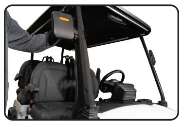
Starting with the passenger or driver side panel, feed piping down track. Pull side panel towards rear until the front zipper is even with the zipper on the front strut cover. Connect and zip all the way down. Repeat on opposite side.
