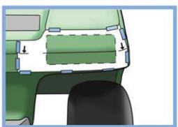
3. Use a marker or other marking device to trace the inside contour of the template.
